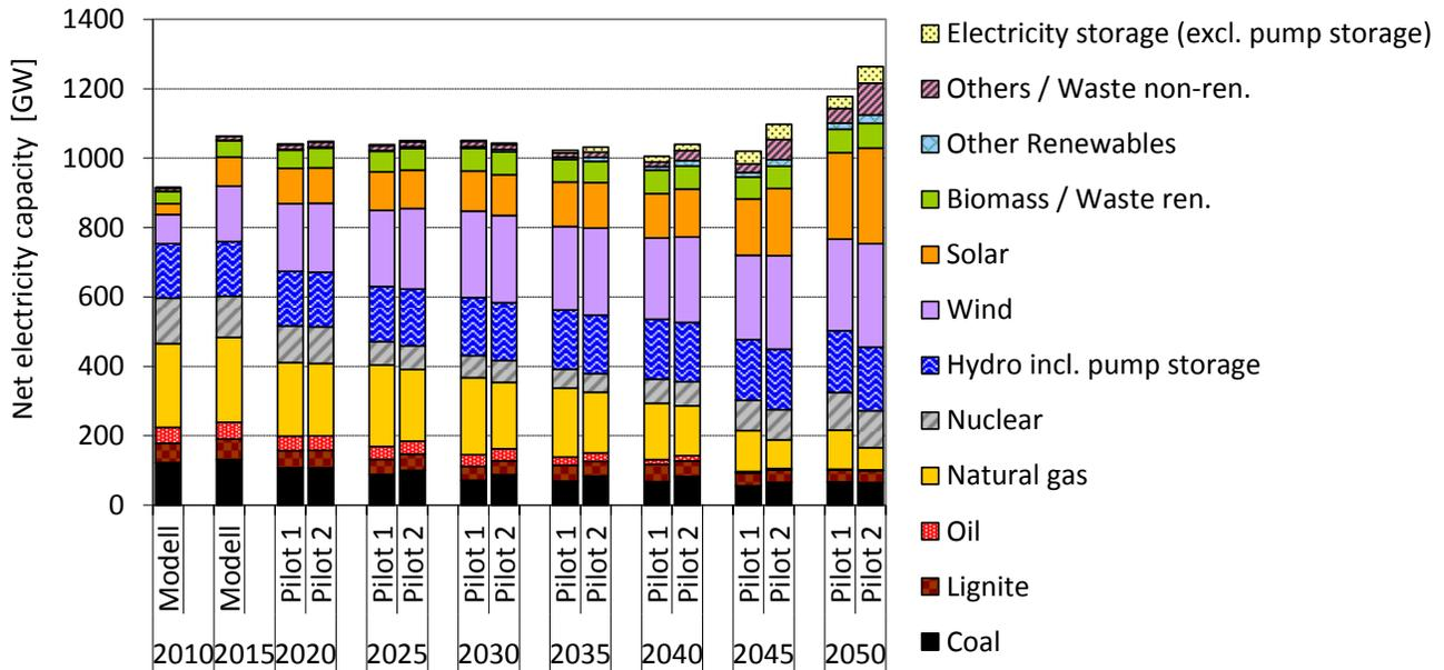
Figure 3. Electrical capacity of power and chp plants in the EU28 in TIMES PanEU.
